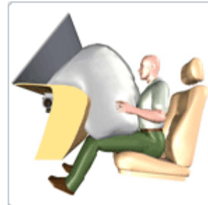
50th percentile male in mid-seat position. Dual-depth airbag deploys to full depth and inflation is at full output.
