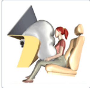
5th percentile female seated in the full-forward position. Dual-depth airbag is at restrained deployment depth and inflation is at low output.
