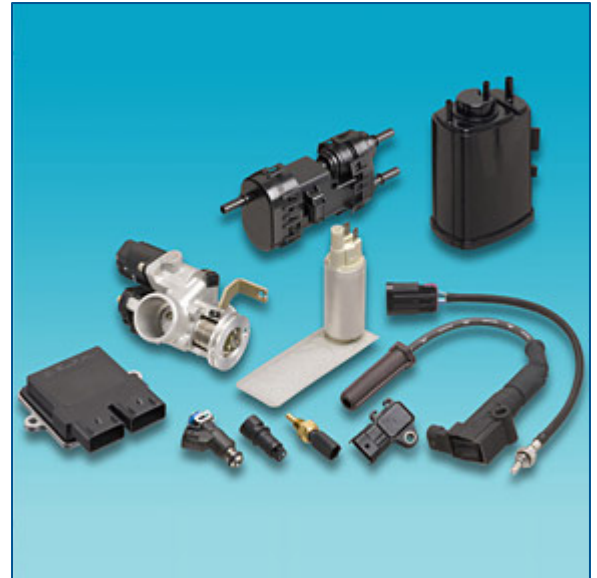
The Delphi Multec ® Electronic Fuel Injection for small engine commercial products includes: (from top right, clockwise) evaporative emissions canister, mini-switching oxygen sensor, ignition coil, manifold absolute pressure sensor, engine temperature sensor, intake air temperature sensor, fuel injector, engine control module, throttle body, fuel module and T-11 Fuel Pump (center).
