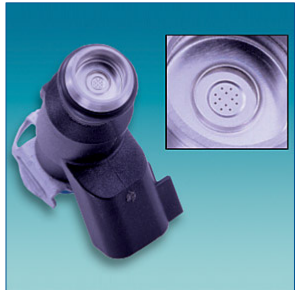
The tip of Delphi Multec® 3.5 Fuel Injectors features a multi-hole director plate that provides fine atomization.
