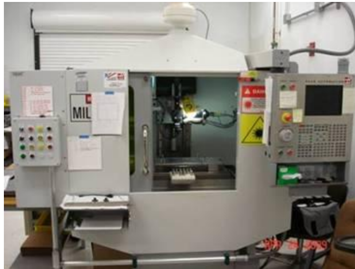
Laser welding of SOFC parts
