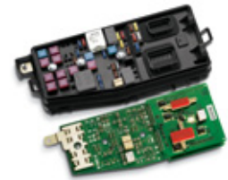
Smart BEC: This is a stamped metal, high-current feed printed circuit board (PCB), with bussing layers and electronics, that supports both centralized and distributed architectures.
