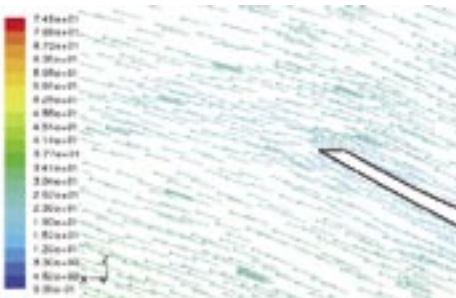
Figure 20. CFD analysis at trailing edge mid blade
