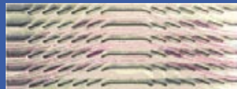
Figure 9. Flow re-alignment through a louvre array - scale model in water channel
