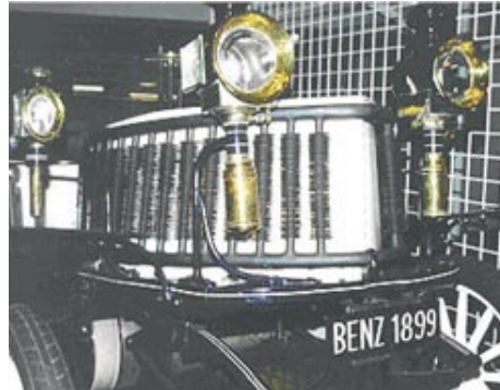
Figure 2. Radiator wrapped around front of vehicle
