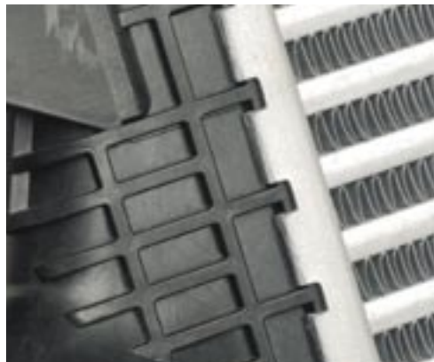
Figure 13. Radiator tank clinched on header
